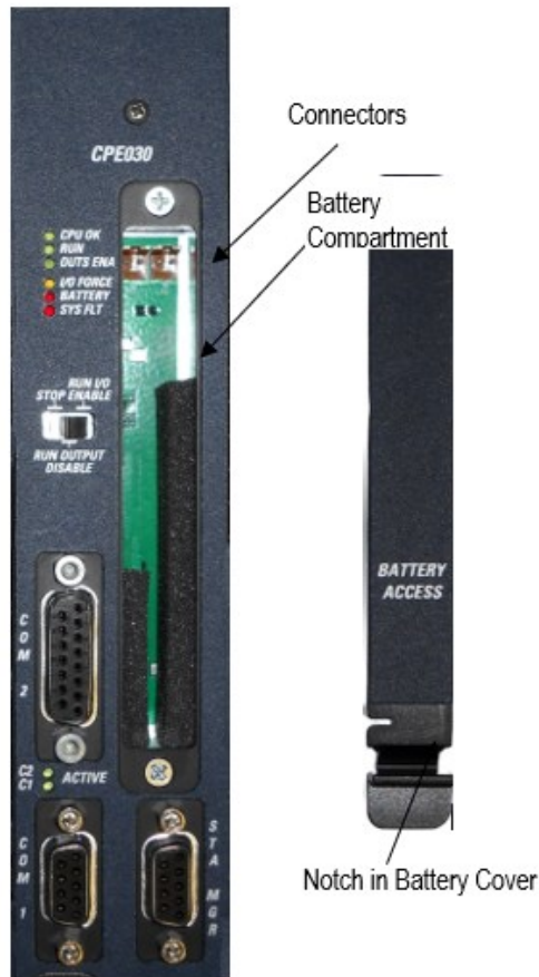
Figure 6: RX7i Battery Installation
