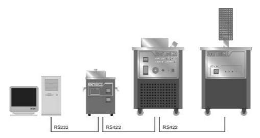
Note: The RS 422 standard specifies a maximum lead length of 1200M (4000ft). A true RS422 port will be required to realise such lead lengths. The Isotech conversion leads are suitable for maximum combined lead lengths of 10M that is adequate for most applications.
