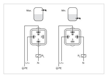
VEGASWING 53 with valve block according to ISO 4400
