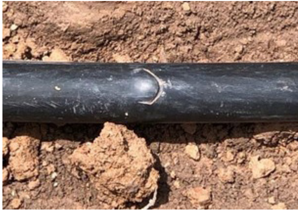
Fig. 7. Damage found in the cable during installation.
