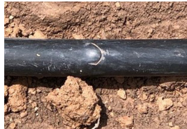
Fig. 6. Damage found in the cable during installation.
