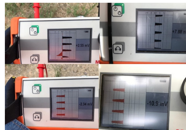
Fig. 3. Pinpointing a fault in buried cable.
