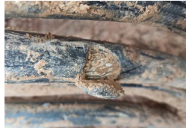
Fig. 5. Damage found in the cable during installation.
