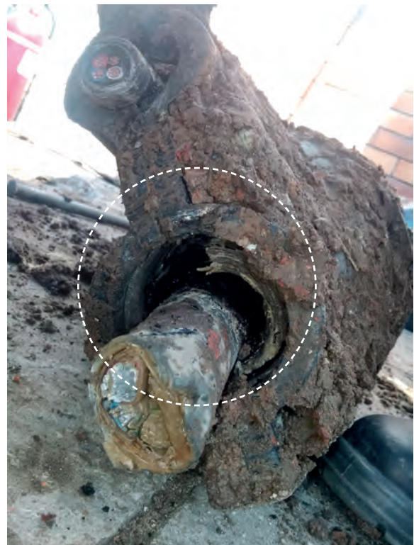
Figure 7: T-splice showing 'trunk' cable and smaller 'branch' cable (feeding house service)
