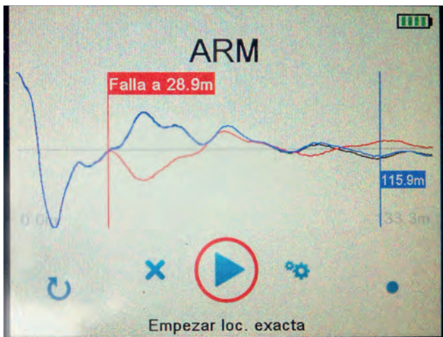
Figure 4: ARM localization of fault
