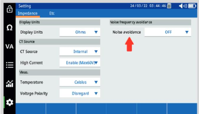
Select "ON" This changes injected frequency. This should have a minimal effect on the measurement but may allow the instrument to better distinguish the signal from the system noise.
