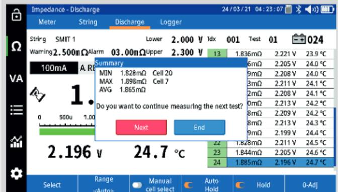
The unit will then prompt the user to either end the test or select "next" to perform the next pass through the string. Press when ready to perform another pass through the string. Press END to end the test.
