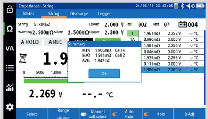
Performing a conductance test on a battery string.
