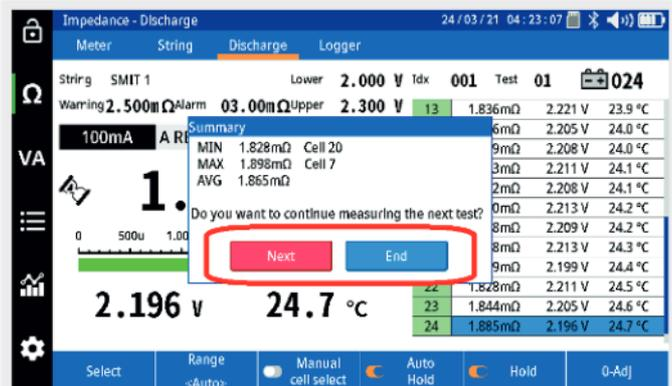
**NOTE :** This value will be associated with the internal impedance changes associated with sulfated plates. It may not correlate with other causes of cell aging such as plate corrosion.
