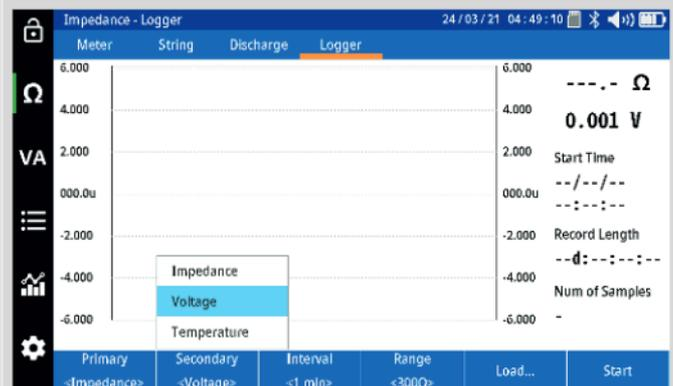
Select "Interval" and then desired recording interval.
