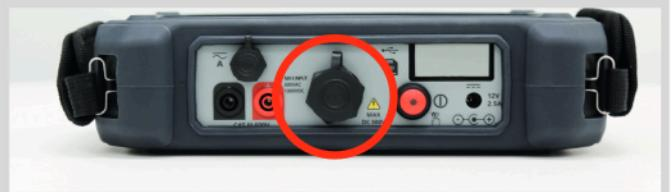
Connect the duplex probes to the BITE5 ADVANCED. to voltage inputs of the BITE5 ADVANCED.
