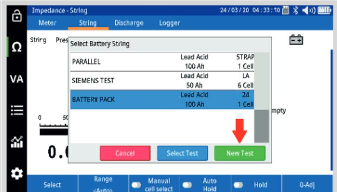
Place the kelvin clips across the battery pack or the battery string. The BITE5 Advanced will automatically take the measurement and save it to memory.
