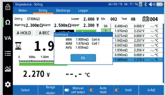
To record the negative terminal connection, close the summary and measure from the end of the negative charger lead to the last post on the last battery. This value will be saved as a strap.
