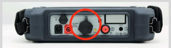
Connect the duplex probes to the BITE5 ADVANCED.
