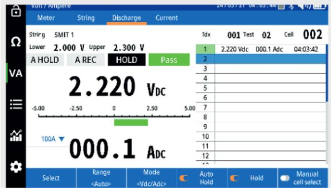
Take measurement of each following cell. Each measurement shall be saved in sequence with a cell number, date, and time stamp.
