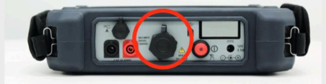
Connect the duplex probes to the BITE5 ADVANCED to voltage inputs of the BITE5 ADVANCED.
