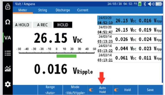
Adding a Ripple (AC) Voltage, Ripple (AC)Current or a Float (DC) Current value to a string.
