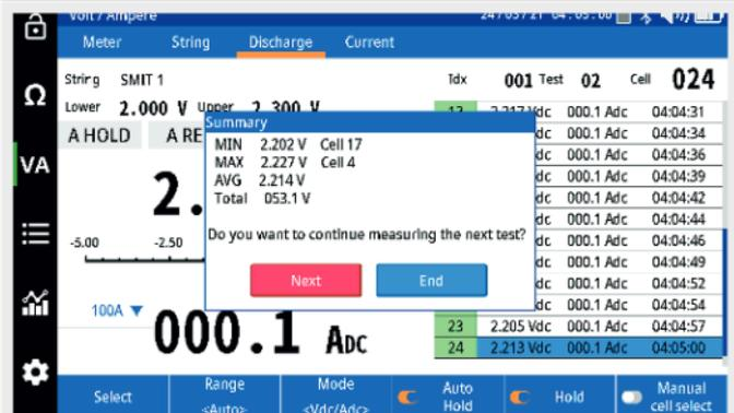
The unit will then prompt the user to either end the test or select "next" to perform the next pass through the string. Press when ready to perform another pass through the string. Press END to end the test.
