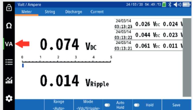
When the VA ICON is selected the BITE5 Advanced will use the banana jack inputs and the current clamp input.
