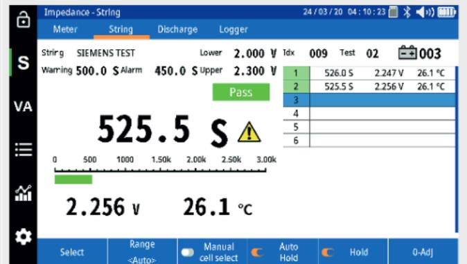
Continue taking measurement of each cell and strap in sequence until you reach the last cell in the string. When the BITE5 ADVANCED measures the last cell in the string, it will display a summary.
