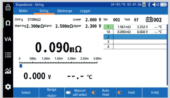
Continue taking measurements until the parallel string is reached. At this point move the AC CT to the path that was just measured and then continue measuring the cells and straps if the parallel string.
