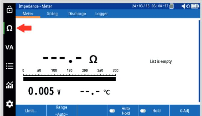
When the Ohm ( $\Omega$ ) ICON is selected the BITE5 Advanced will use the Duplex input.
