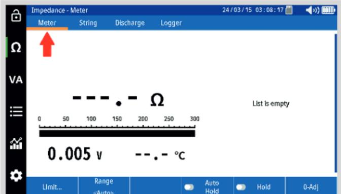
Select "Limit" if you would like to program impedance and voltage limits for the measurement.
