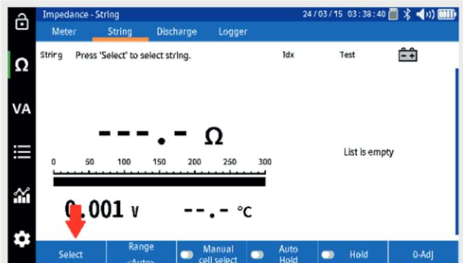
Performing a NERC terminal mode impedance test on a battery string.
