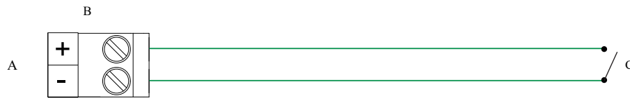
Figure 2-29: Discrete Input Wiring (Internally Powered)
